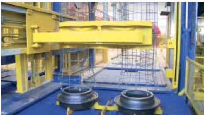
Fig. 5 Pallet and cage handling fully automated.
