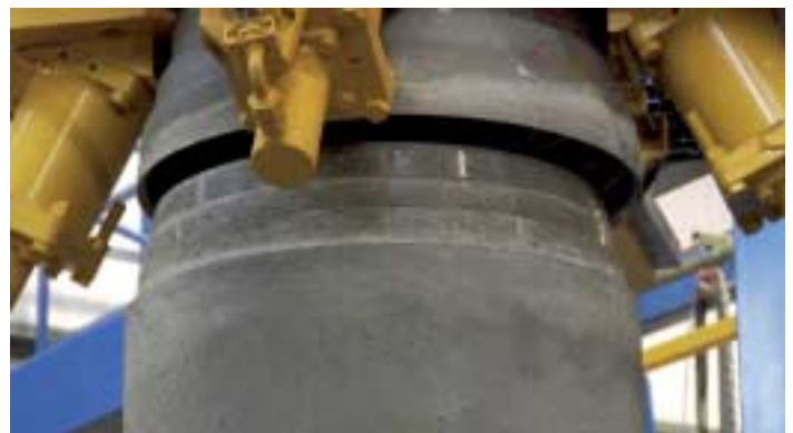
Fig. 2 State-of-the-art-production with steel top pallets.
