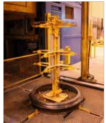
Before the production of the manhole risers starts, the pallets, the hoops, the lifting anchors and step rungs are automatically positioned.
