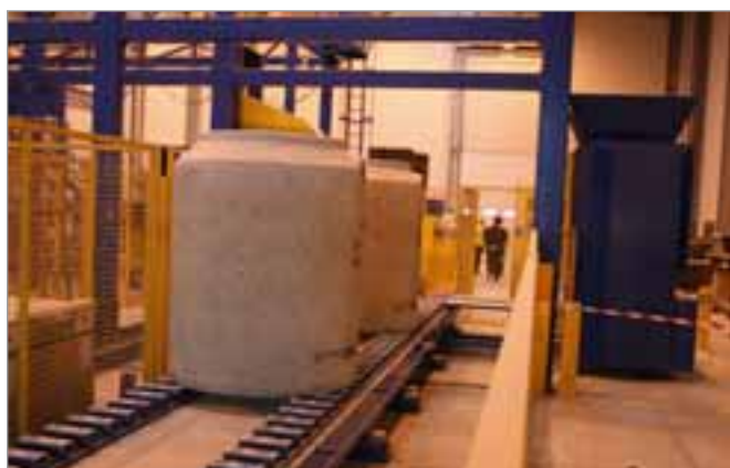
The plant disposes of a fully automatic pallet handling system.
