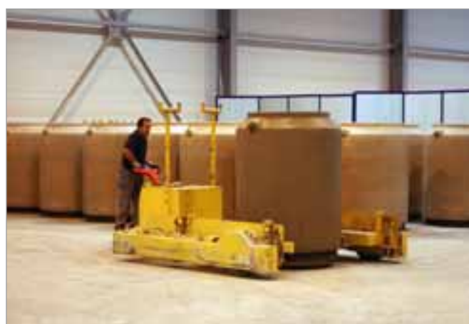
An electrical transporter transfers the manhole components to the curing area.
