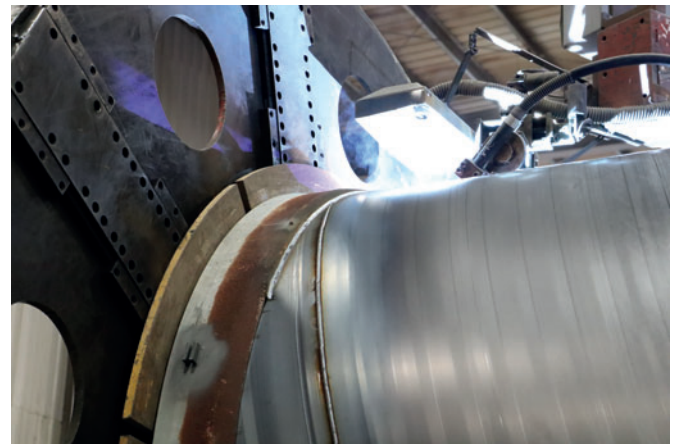
The end rings are then welded, over the entire periphery of the steel cylinder in order to be coupled and sealed.
