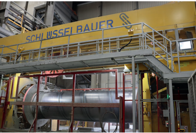
The high-speed pre-stressing machine from Schlüsselbauer Technology has been integrated into the production line, significantly improving the process.
