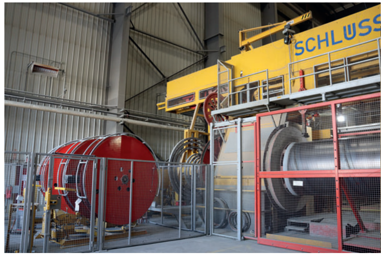
The high-speed pre-stressing machine from Schlüsselbauer Technology has been integrated into the production line, significantly improving the process.
