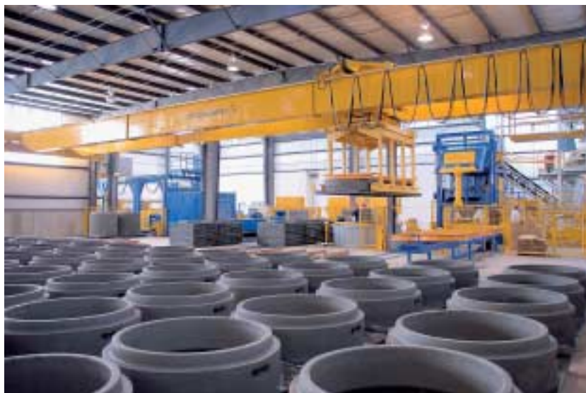
Fig. 4 Fully automated handling of any type of manhole components.
