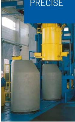
Production system for manhole components as well as reinforced and non-reinforced concrete pipe, road side channels, and pipe connection parts
