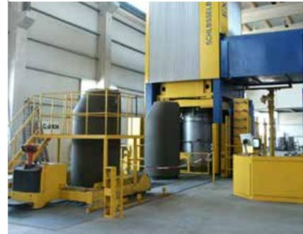
Modular, fully automatic production system for concrete pipe and manhole components
