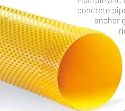
The pull-out strength of each anchor is more than 250 N (56 lbs.); the entire liner can safely withstand permanent groundwater pressure of at least 1.5 bar (22 psi). Even large temperature fluctuations will not cause the liner to separate from the surrounding concrete. Liners can be produced in varying material thicknesses 1.65 to 3 mm (0.065 to 0.12 inches) to accommodate different regional, standard- or project-specific requirements.
