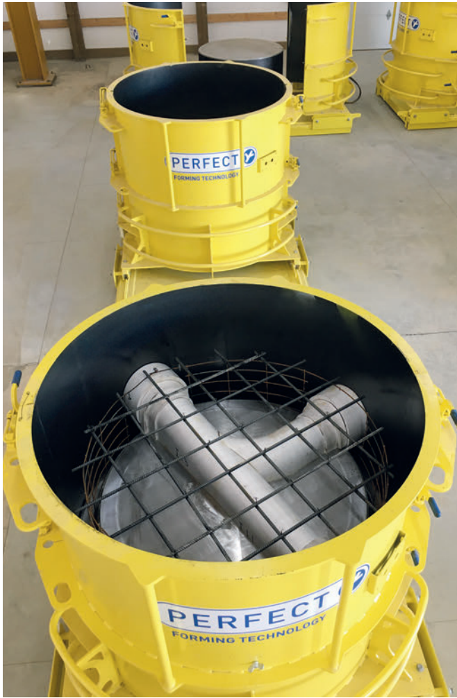
Perfect Forming Technology - this term refers to the casting moulds for high-quality concrete components that are constantly being optimized by Schlüsselbauer Technology
