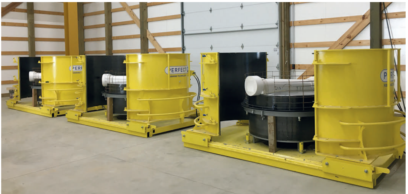
The casting moulds that have been prepared with EPS channels and steel reinforcement are ready to be filled with self-compacting concrete
