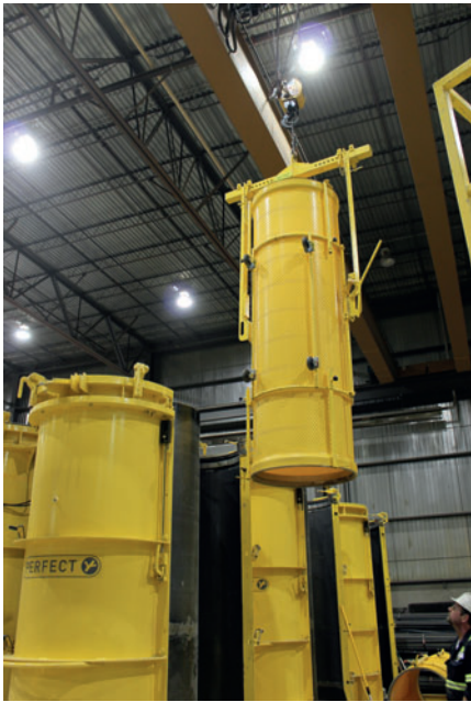
A crane transports the formed liner (with pallets) to the formwork mold and sets it down over the shrinkable mold core
