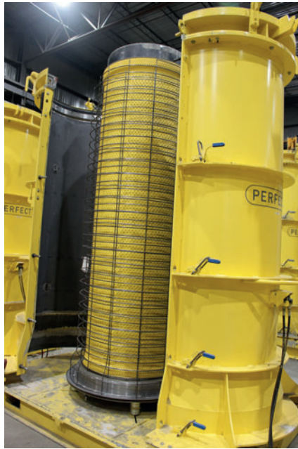
Fully prepared with liner and reinforcement cage
