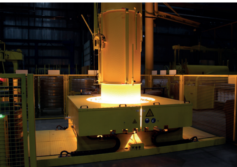
Forming pipe joints in the reshaping station
