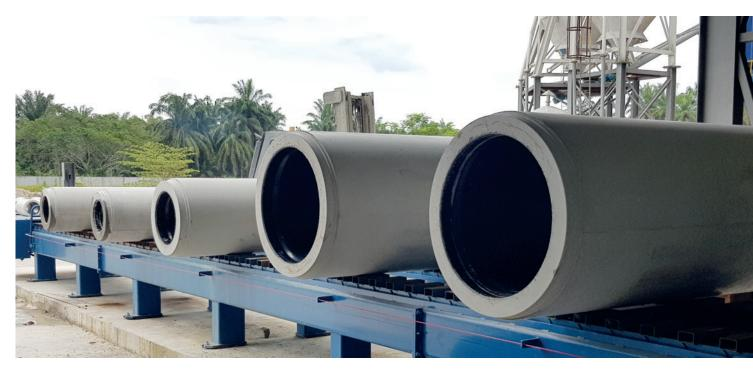
At Bilcon Industries Perfect Jacking pipes are manufactured up to a nominal width of DN 900.
