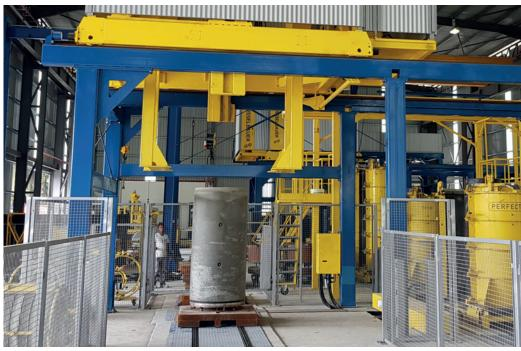
After hardening in the mould, the jacking pipes get demoulded.
