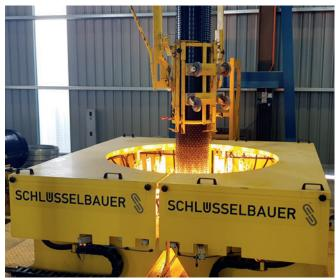
Here, both ends of the liner will be formed in a thermoplastic process according to subsequent pipe joint.
