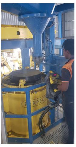
Filling the prepared moulds with self-compacting concrete
