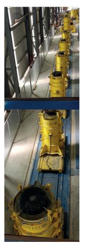
The filled formwork is on the way to the hardening station
