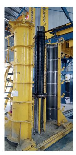
Fully prepared moulds with Perfect liner and reinforcement cage
