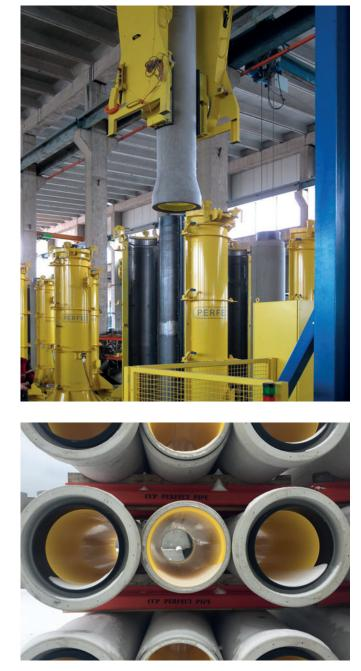
Elsewhere, plastic pipes are increasingly being built into concrete or liquid soil—as a concrete pipe with firmly attached HDPE corrosion protection, Perfect Pipe brings added value back into concrete production here.
