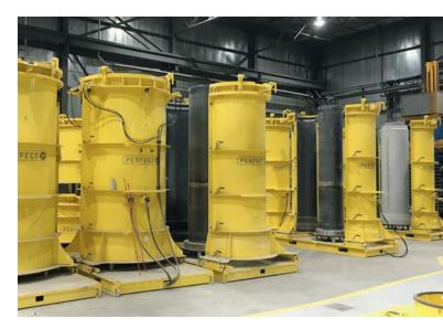
The Perfect Forming Technology concept is suitable for all kinds of infrastructure components, including pipes, manhole components or other components of a similar geometry.
