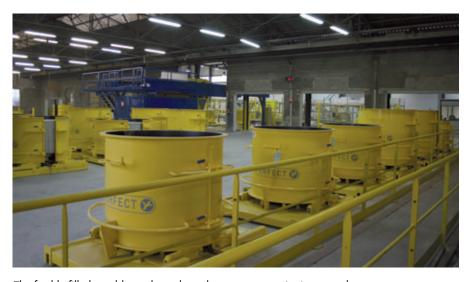
The freshly filled moulds are brought to the storage area in tipper trucks
