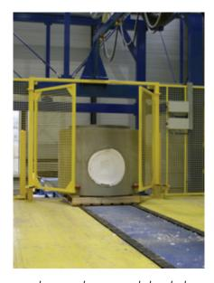
...and set onto the conveyor belt to the last processing station, in which the EPS mould bodies are removed from the manhole bases.
