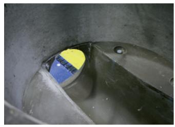
Finished manhole base before it is transported to the external storage area
