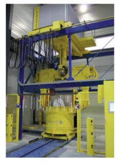
The hardened manhole bases are removed from the open mould with the gripper of the crane rail....
