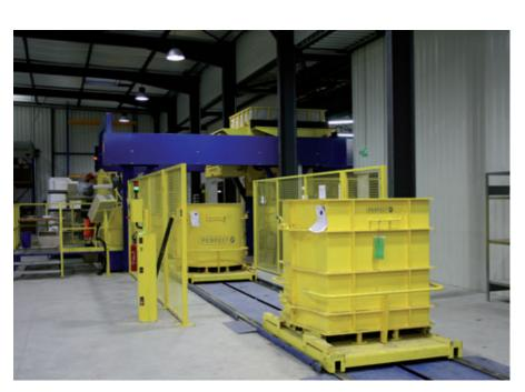
The prepared moulds drive automatically into the casting station
