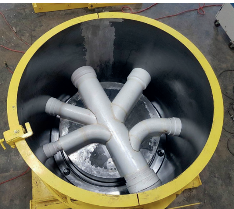
Efficient procedure for the production of custom-made concrete manhole bases: negative channel from composite EPS moulded parts.
