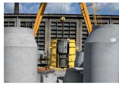
After sufficient hardening time, the moulds are opened again and the manhole cones are carefully lifted by crane out of the mould
