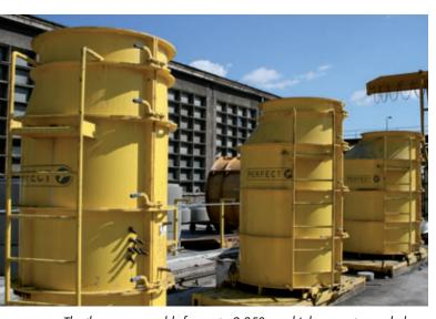
The three new moulds for up to 2,350 mm high concrete manhole cones with nominal widths of 1,000, 1,200 and 1,500 mm
