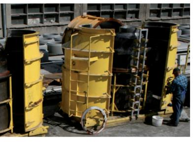
A special template is hung on the mould core for the exact setting of the bushings for the steps
