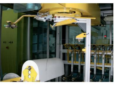
The individual negative channel runs made of EPS hard foam are produced with modern sawing technology (here 3D hot wire saw)
