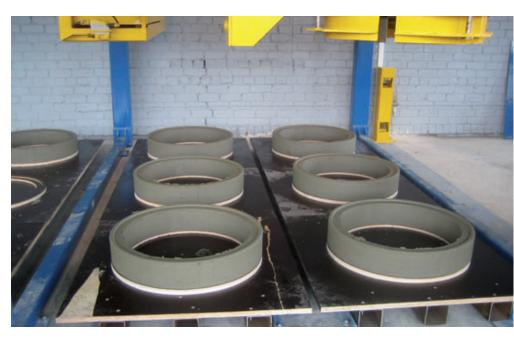
Adjustment ring with rebated joint DN 700 from the Ringmaster production at the company JSC Gelgaudiskio Gelzbetonis
