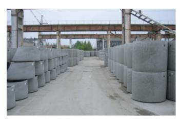
Modern manhole components for use in civil engineering in Lithuania -This photo shows manhole cones and manhole rings at the company Kauno Gelzbetonis.
