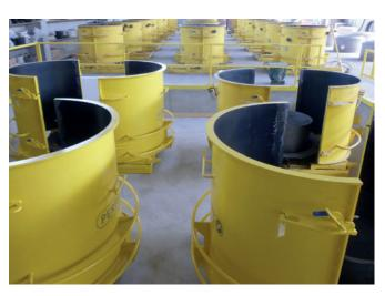
User-friendly steel moulds for manufacturing wet-cast concrete components with individually customised channel configurations.
