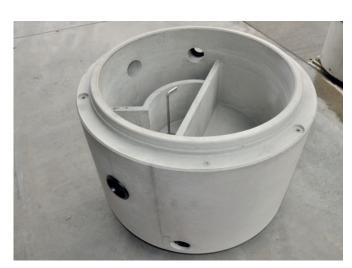
DN1200 water chamber manufactured from flowing concrete with individually moulded channel and gaskets encased in concrete.
