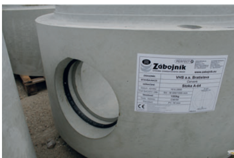
At the second company site, Perfect concrete manhole bases are produced with tailor-made channels and, in most cases, integrated gaskets.
