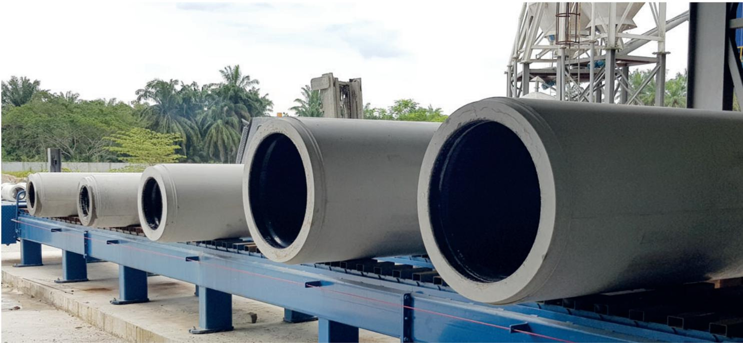
At Bilcon Industries Perfect Jacking pipes are manufactured up to a nominal width of DN 900.
