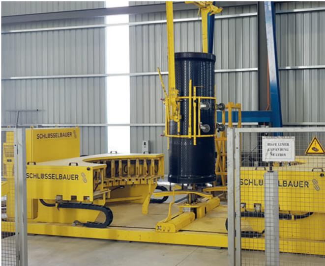
The welded liner cylinder will be transported with an auxiliary structure and the crane to the reshaping station.
