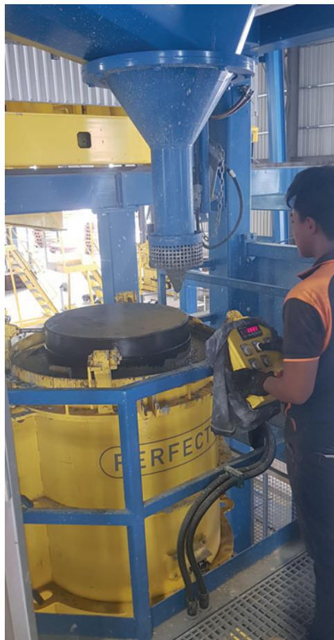
Filling the prepared moulds with self-compacting concrete
