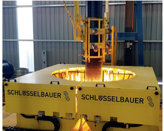
Here, both ends of the liner will be formed in a thermoplastic process according to subsequent pipe joint.
