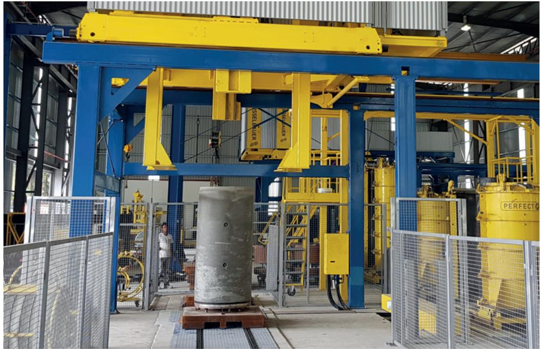
After hardening in the mould, the jacking pipes get demoulded.
