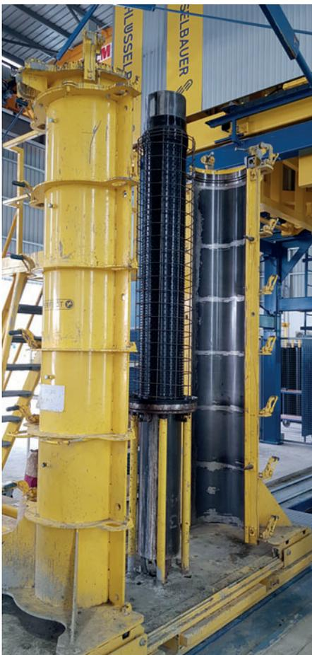
Fully prepared moulds with Perfect liner and reinforcement cage
