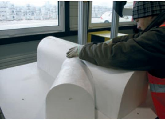
*The individual cut sections are put together, the channel courses shown by a laser projection help to correctly position the moulded parts*
