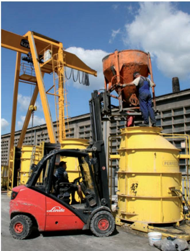
*Concreting is done with a forklift and concrete bucket; as with the Perfect System, only self-compacting concrete is used*
