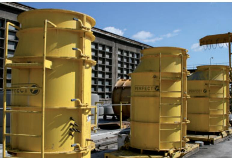
The three new moulds for up to 2,350 mm high concrete manhole cones with nominal widths of 1,000, 1,200 and 1,500 mm
