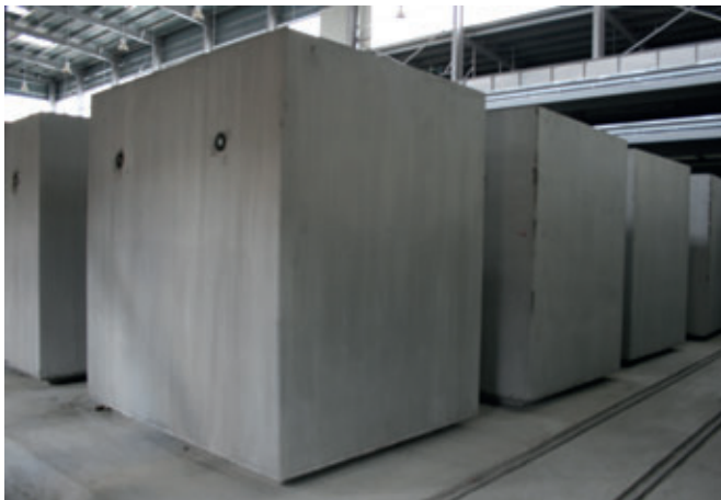
Large-format frame components with 2000 x 1500; 2000 x 2000; 2000 x 2500 and 2500 x 2500 mm dimensions are produced on an industrial scale at Amiantit Oman Concrete Products LLC.
