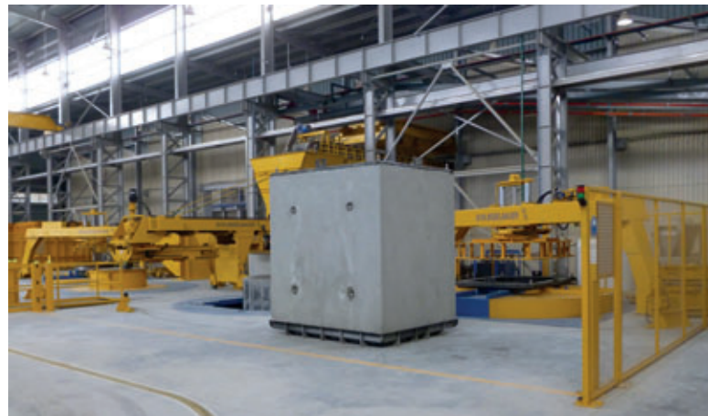
By using steel set-rings, the Exact XL plant permits precisely manufactured joints on all products – pipes and frame components.
