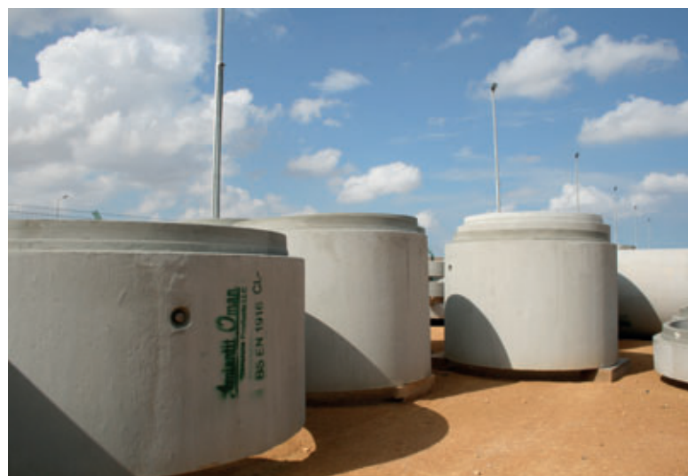
Even large format manhole components are manufactured on the Exact XL production line.
