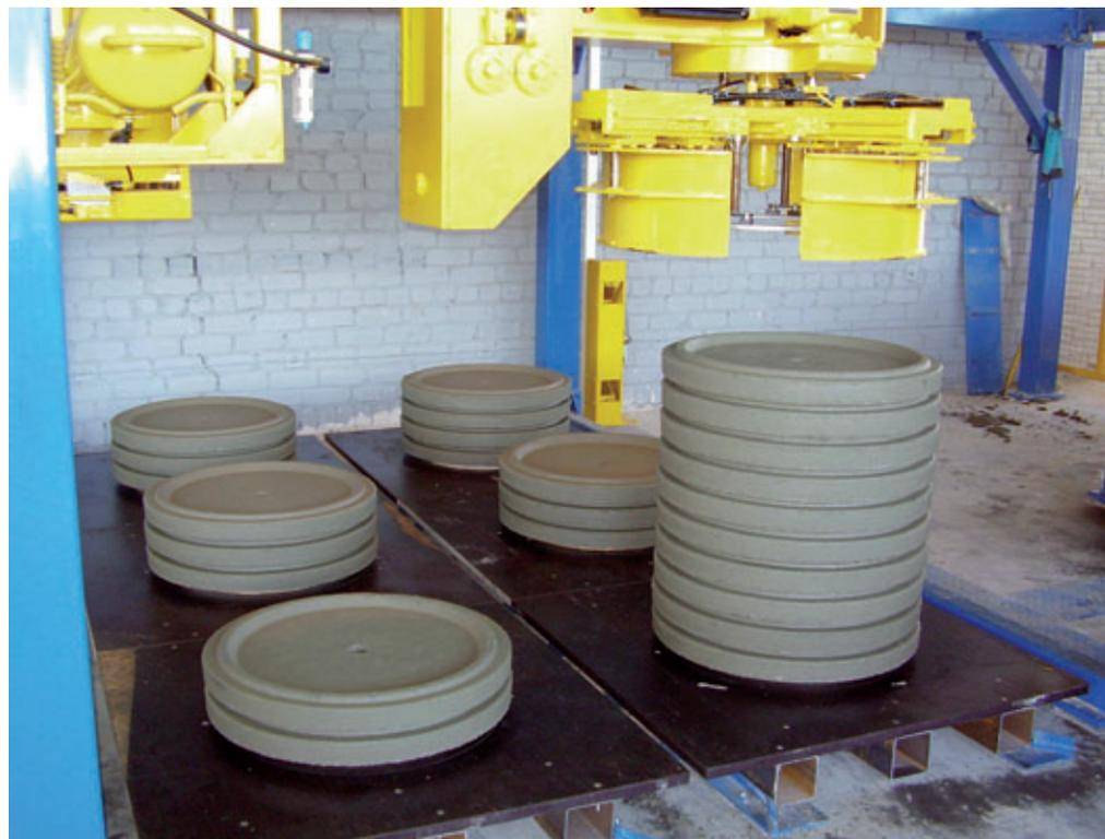
Production and handling of covers by use of the Ringmaster automatic stacking system.
