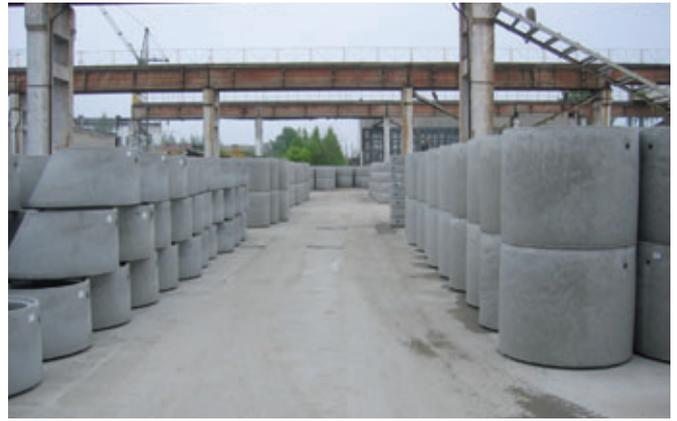
Modern manhole components for use in civil engineering in Lithuania -This photo shows manhole cones and manhole rings at the company Kauno Gelzbetonis.
