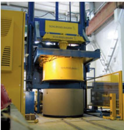
Production of manhole rings with different dimensions at the concrete works Kauno Gelzbetonis and Vilnius Gelzbetoninis Konstrukcijs Gamykla Nr. 3.
