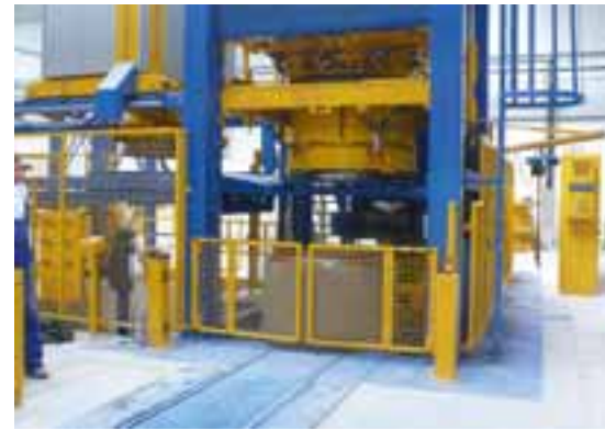
The Exact 1500 in operation – fully automatic production of manhole risers with top and bottom pallets
