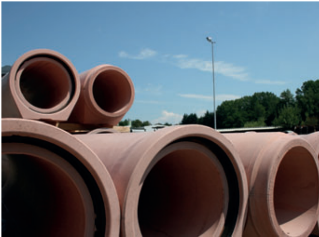
Even pipes in nominal width classes 2 and 3 are now manufactured as prebed pipes – DN800 concrete base pipes are shown in the image
