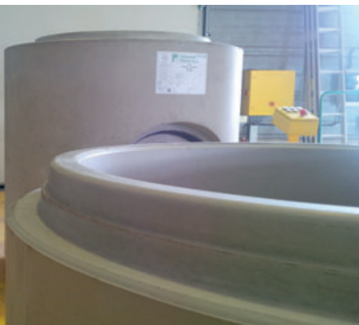
Immaculate concrete surfaces, including the spigot end.
