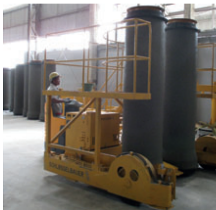
The second member of personnel responsible for pipe production moves the freshly-made products to the curing area, using a removal truck.
