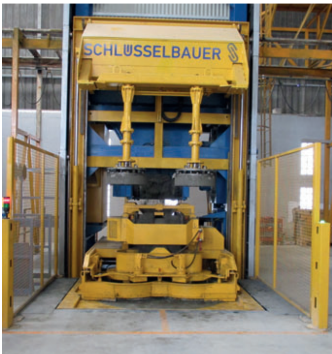
Two moulds can be fed with concrete simultaneously thanks to a conveyor belt and the corresponding filling unit.
