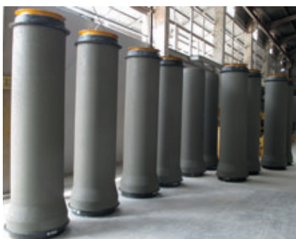
The concrete pipes usually remain for one working day in the curing area.
