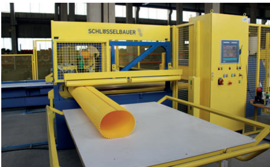
Liner is welded to create a water-tight cylinder in a fully-automated process.
