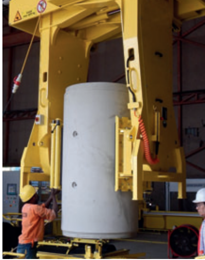
Secure product handling with a hydraulic gripper
