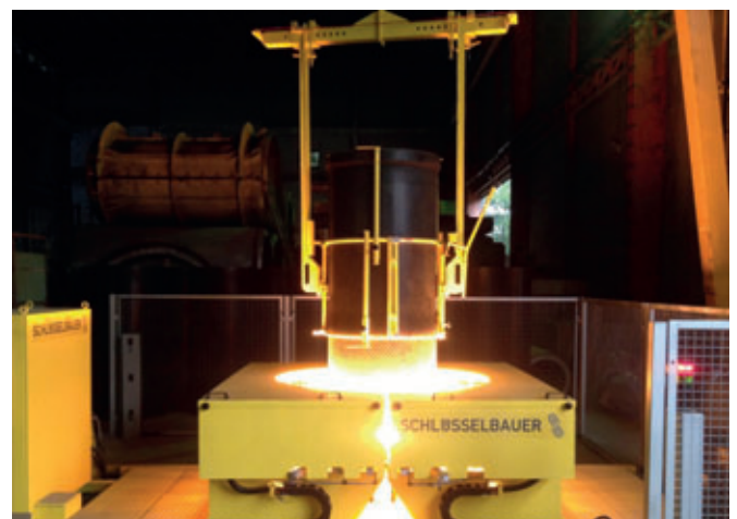
Thermoplastic forming of the Perfect Liner ends for the future connector position
