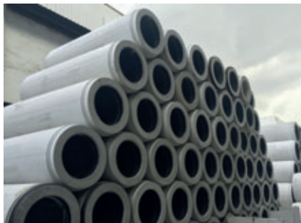
Storage of ready jacking pipes at Bilcon Industries in Singapore
