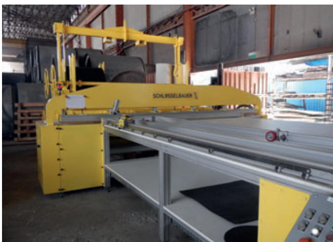
Fully automated cutting and welding of the Perfect Liner film according the requested nominal width
